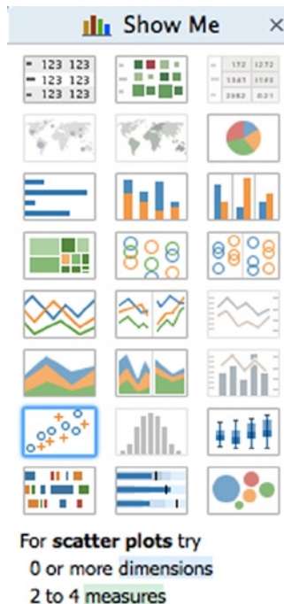
Figure 5-5. The Show Me popup in Tableau Desktop allows users to switch easily between different kinds of visualizations (Courtesy Tableau Software; used with permission)
